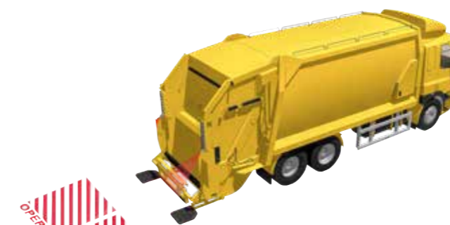
Demarcating a work area
